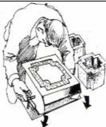
With a multi-use steel mould, after vibration a worker can immediately release the product after vibration to set and cure on the ground.
