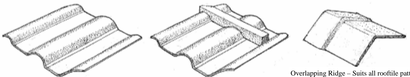
Standard Semi Sheet – 4 cover 1 square metre. Top Row Semi Sheet (infill block fits under ridge).
