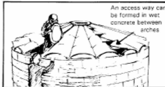
8. Access to the interior is through the centre manhole which has a removable concrete cover.
