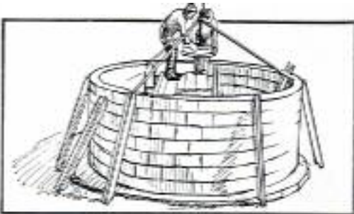
4. The roof structure is assembled by suspending the centre manhole ring from the tripod jack and placing beams in position.
