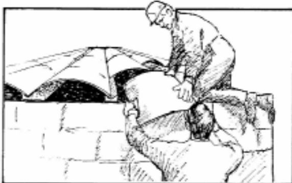
7. The arch elements fit into the grooves on the beams. The end stops are mortared in position.
