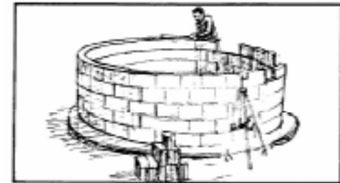
3. Build up tank row by row mortaring into place until desired height is realised. Plaster the inner surface to seal against leakages.
